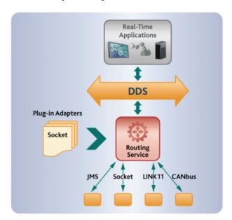
Quickly build and deploy bridges between natively incompatible protocols and technologies using RTI Data Distribution Service.
