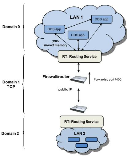
You will run two copies of *RTI Routing Service*. One copy will run on a machine that is behind a firewall/router with a public IP (First Peer); the other will run on a machine in another LAN (Second Peer).
