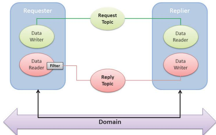
*Requesters* and *Repliers* are built on top of DDS. There are APIs in C, C++, Java and C#; these APIs have been designed to be closer to the programming language. In particular, the C++ and Java Request-Reply APIs include significant improvements with respect to the traditional DDS API, such as the use of generic code (templates in C++ and generics in Java) or close integration with standard language features and utilities (like the C++ STL, and Java Collections).
