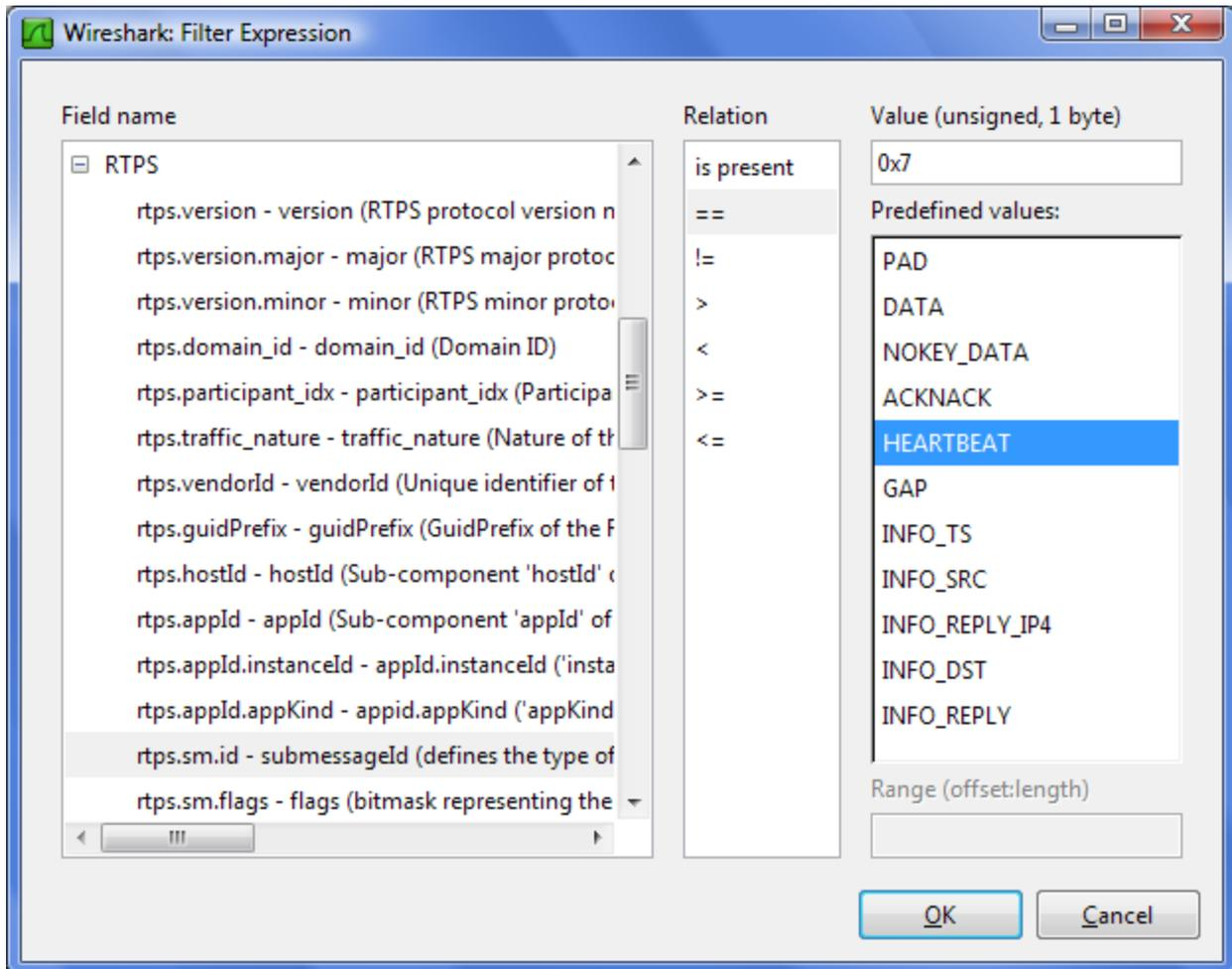
Figure 5.3 Filtering by Submessage Type
