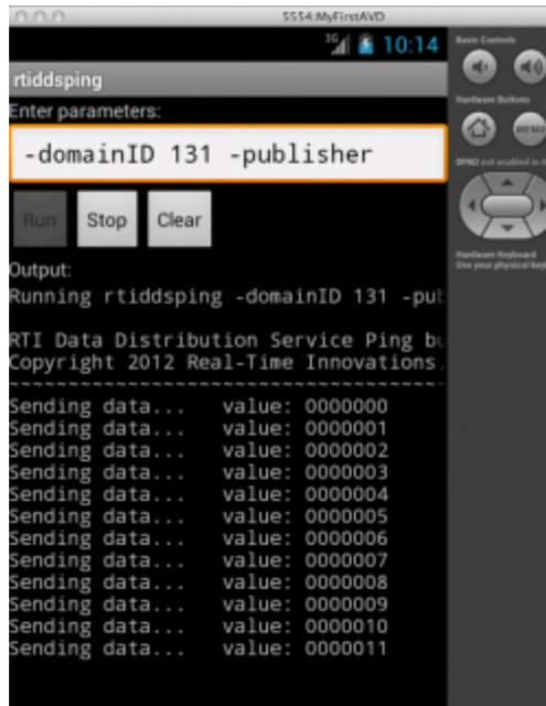
4. Note that the **Run** button will be disabled until the Ping process is finished (i.e., if you have specified (in the parameters) a **-numSamples** value with the publisher, or a **-timeout** value with the subscriber). To stop a running Ping process gracefully, click or touch the **Stop** button. Once the ping process is finished, the **Run** button will be enabled again.
