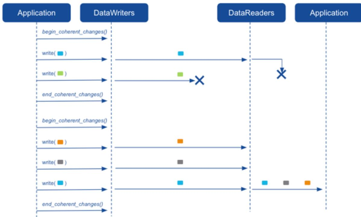
By default, the first coherent set was not provided to the application because it was deemed incomplete by the DataReaders. (Different colored rectangles represent samples from different Topics.) The second coherent set was received completely by the DataReaders, and was therefore provided to the application.
