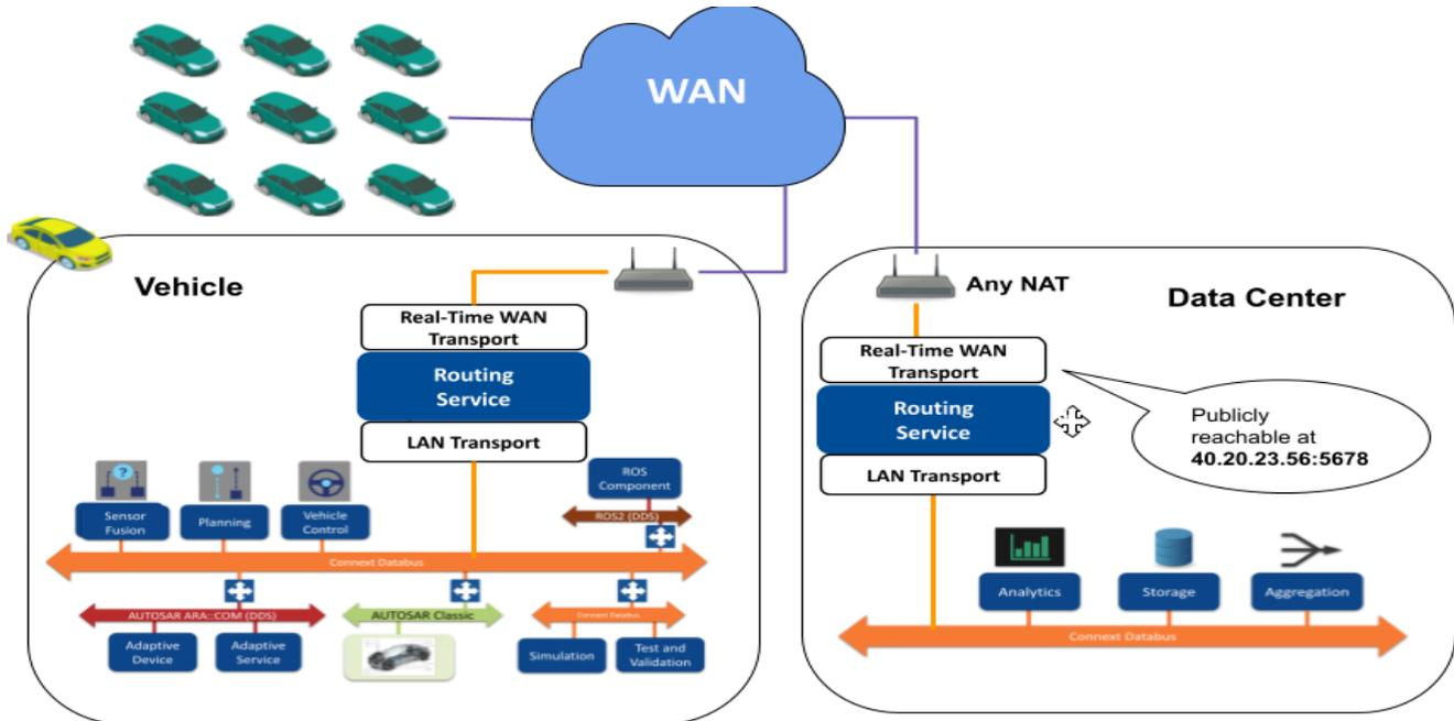
*An example scenario of an Edge-to-Data Center deployment for a fleet of vehicles using a Routing Service in the vehicles and in the data center. This is one of the many deployment configurations that RTI Real-Time WAN Transport supports.*
