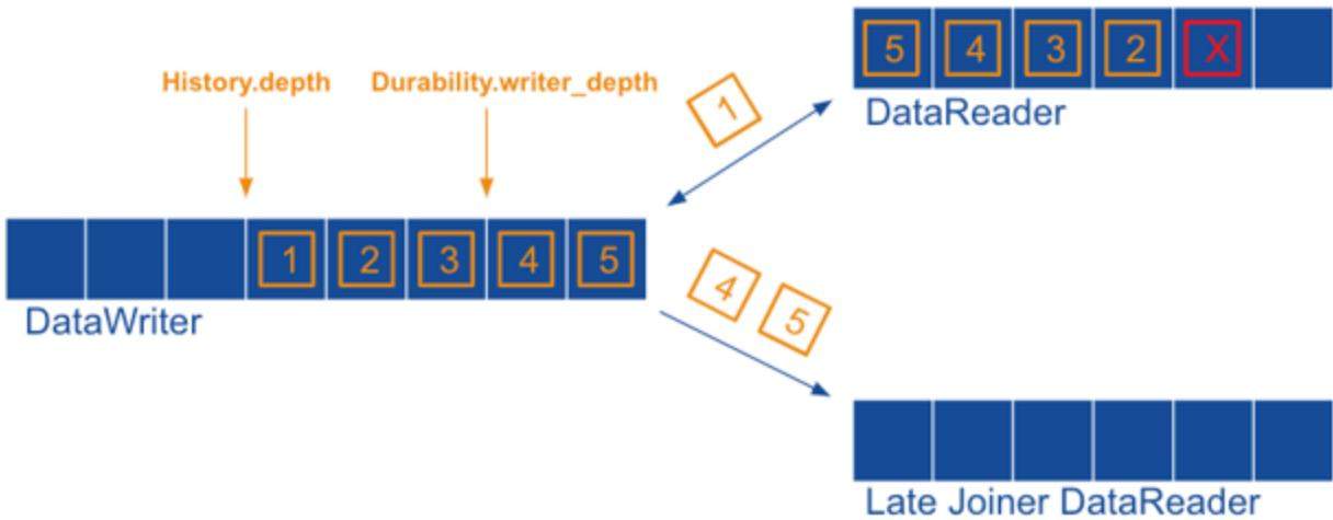
*While a History.depth of 5 samples is maintained to repair losses for DataReaders that haven't acknowledged the samples yet, Durability.writer\_depth is set up to send only the last two samples to late-joining DataReaders*
