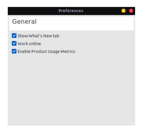
The **Preferences** settings are stored in the file **launcher.properties**, in **rti\_workspace**/*version*/user\_ **config/launcher**.
