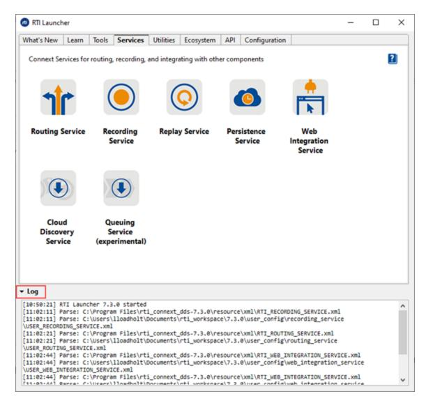
Log files: Launcher logs output and errors to files in a special directory. This directory can be found in the user home's RTI workspace directory: rti\_workspace/<version>/user\_con-fig/launcher/logs. Launcher's execution log files are named with the following pattern: launcher-log-<timestamp>.txt. Every execution of Launcher creates a different log file.
