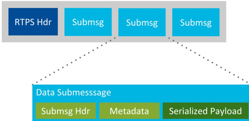
Figure 8.2: Structure of an unprotected RTPS packet.
