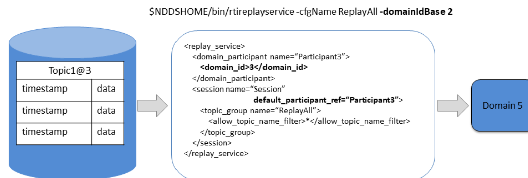
Figure 5.4: To replay data in a different domain than where it was recorded, use the -domainIdBase command-line parameter to specify a base ID for the replay domain. Here, by specifying a domainIdBase of 2, all Topics will be replayed in their original domain, plus 2.
