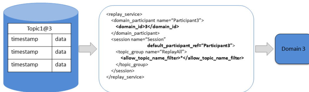
Figure 5.3: The domain ID specified inside a DomainParticipant, in combination with the Topic name, is used to load data from recorded tables. In this case, the DomainParticipant’s domain ID is set to 3. The topic_group specifies all topics.
