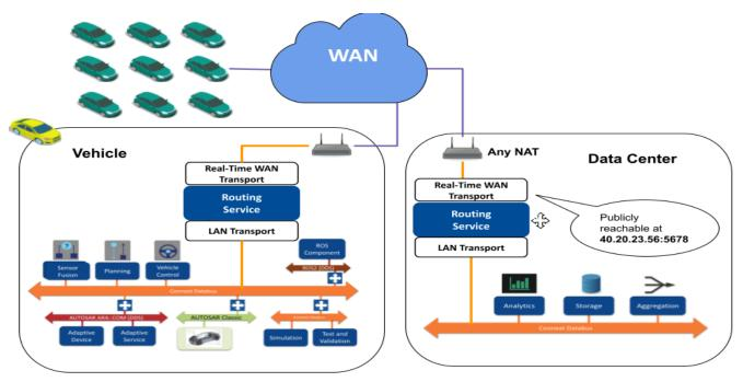
An example scenario of an Edge-to-Data Center deployment for a fleet of vehicles using a Routing Service in the vehicles and in the data center. This is one of the many deployment configurations that RTI Real-Time WAN Transport supports.
